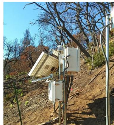
*USGS rainfall/soil moisture gage that was recently installed for the CZU burn scar above Boulder Creek. Ownership of the equipment will transfer to the County following initial technical support and maintenance*
