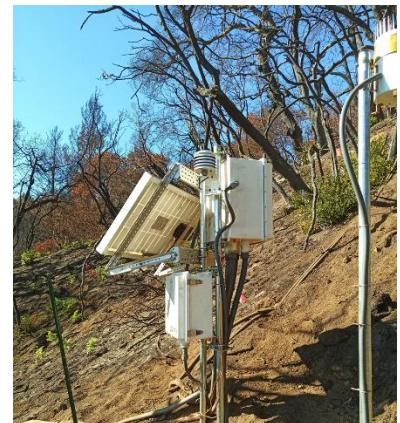
*USGS rainfall/soil moisture gage that was recently installed for the CZU burn scar above Boulder Creek. Ownership of the equipment will transfer to the County following initial technical support and maintenance*
